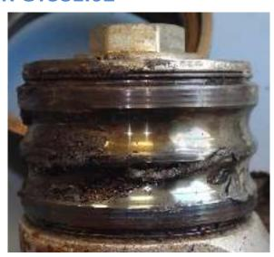
The heat transfer comes from the rear of the belt (which has melted due to the friction) through to the pulley, causing an increase in temperature, which rapidly destroys the grease and bearing cages. This results in the destruction of the tensioner pulley.
