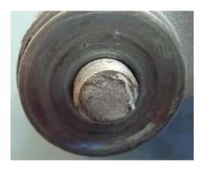
The play that is then created between the roller and the engine causes a belt tension fault, as well as a misalignment of the belt.
