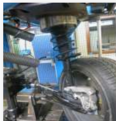
Suspension test bench at the NTN-SNR Test Centre
