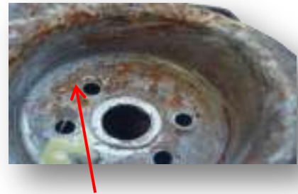
Corrosion caused by movement of the spring
