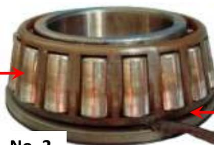
Damaged seal detached from its raceway groove
