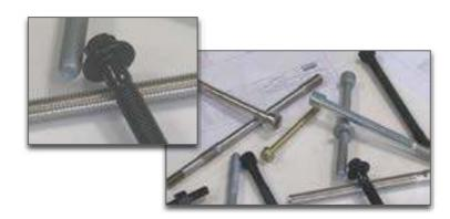
The main function of the cylinder head bolt is to apply the clamping force evenly across the different engine parts involved, usually cylinder block and head, with a capacity to hold it steady ensuring proper sealing of liquids and gases in the cylinder head gasket, withstanding temperature variations, vibrations and positional changes which occur in the engine during operation.
