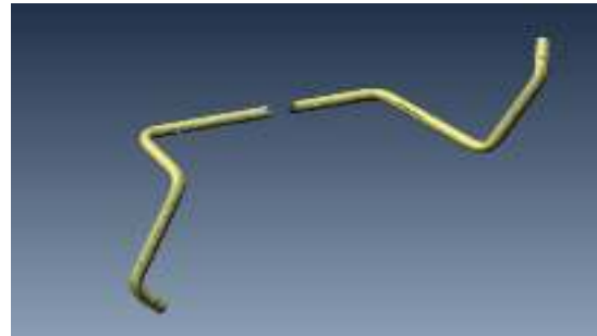
Picture 3. Point cloud of an oil pipe.
