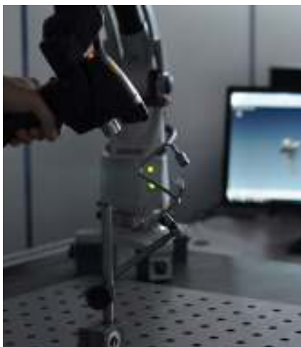
Picture 2. Oil Pipe 3D Scanning.
