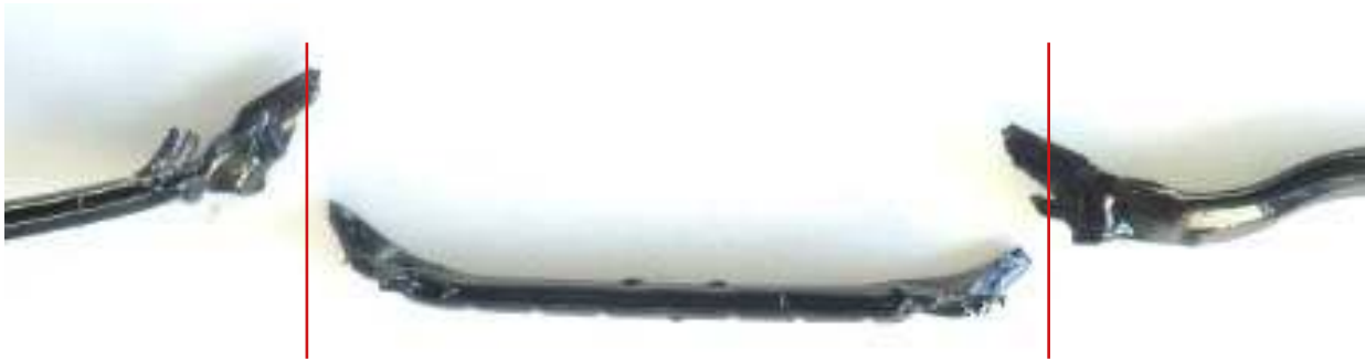
Gasket sectioned by the cover, due to improper positioning during assembly
