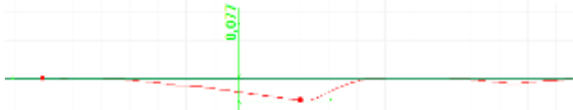
Profile of the contact surface between the seal and the shaft where it's observed wear generated by the sealing lip (mm)
