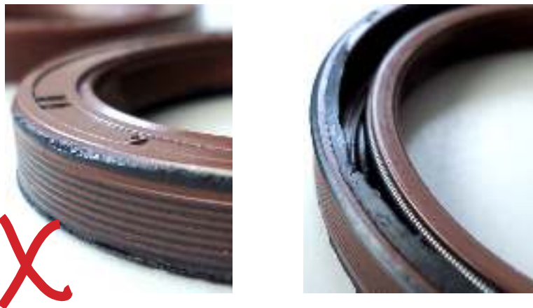
Sealant remains in the external diameter of the seal
