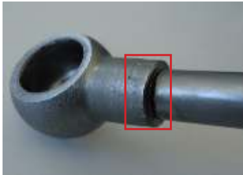
Example of fatigue rupture in the banjo-pipe junction area
