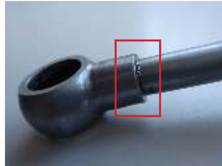
Example of fatigue rupture in the banjo-pipe junction area
