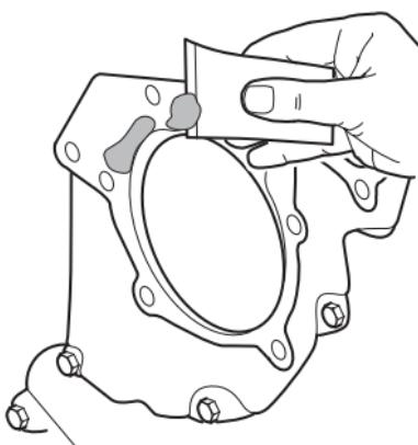
**EN** To fit the water pump only use the sealant supplied with it. Observe the manufacturer's specifications. Use silicon sealants only moderately.
