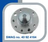
The external diameter of the wheel hub in the cap receptacle is now 57mm instead of 47mm. The old cap can therefore no longer be used.
