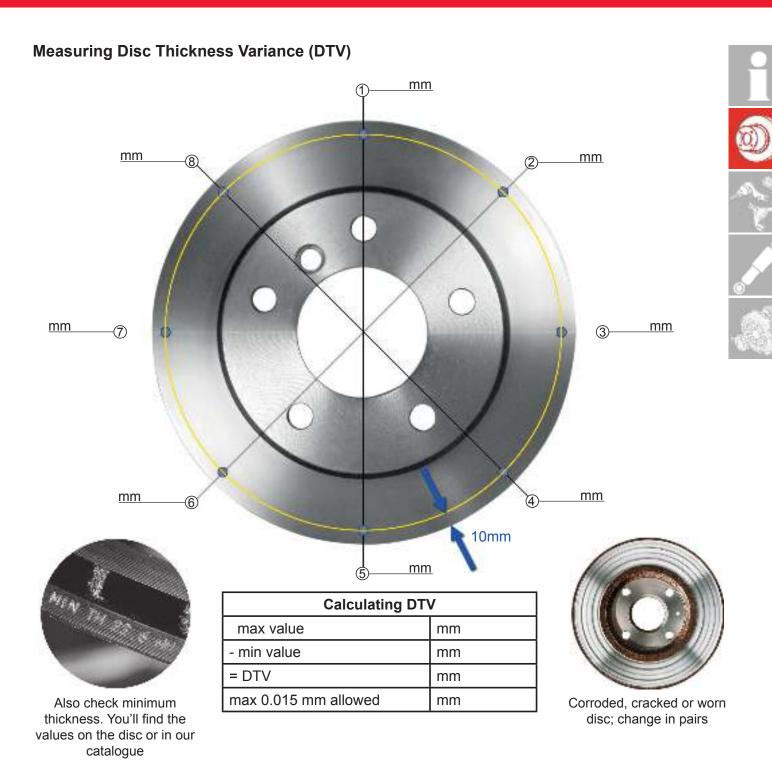
Tool = micrometer screw. Measure eight evenly spaced radial locations on the disc 10 mm from the outer diameter.
