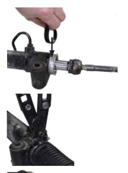
Depending on the model of the steering gear, seals are enclosed.
