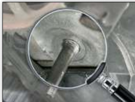
Image 1: The stud is not correctly screwed in.
