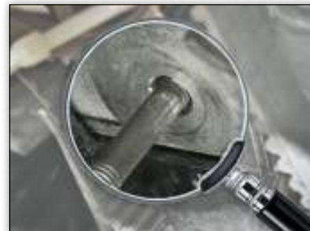
Image 2: The stud is correctly screwed in.
