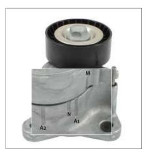
Image 2: Modified markings for the working area of the tensioning arm.
