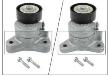
Image 1: Tensioning arm 534 0325 10 – Left, old version with fixing screws M8x40. Right, new version with fixing screws M8x30.
