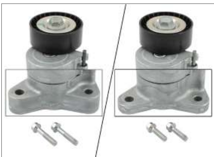
Image 1: Tensioning arm 534 0325 10 – Left, old version with fixing screws M8x40. Right, new version with fixing screws M8x30.
