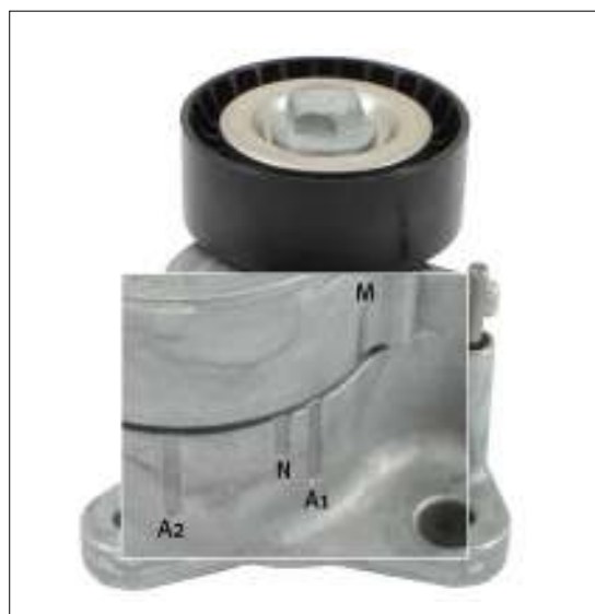
Image 2: Modified markings for the working area of the tensioning arm.
