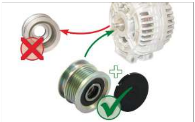
Image 1: Changing from a rigid belt pulley to an over-running alternator pulley
