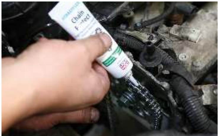
Photo 2: Schaeffler Chain Protect is applied to all timing chain system components during chain installation.
