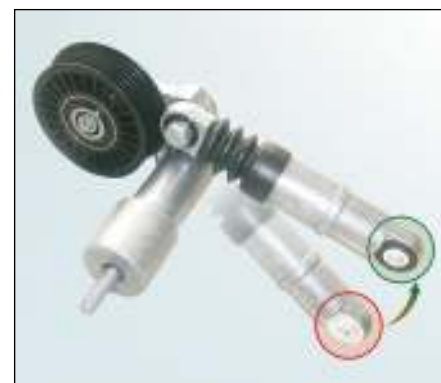
Figure 2: 534 0014 10 - Version showing both black and white plastic bushes on hydraulic damper
