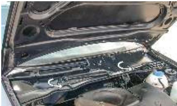
(EN) Remove the filter housing
