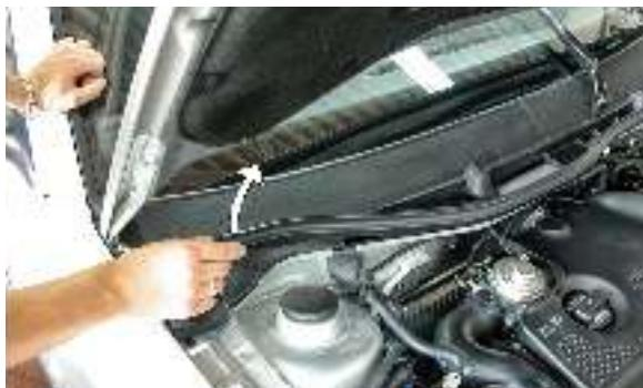
**(EN)** Remove the rubber seal
