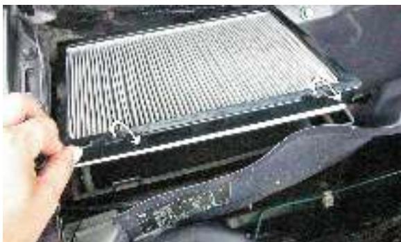
(EN) Unlatch the filter with the frame from its socket. Remove the old filter, insert the new one and carry out the opposite to all the previous operation at the reversed order
