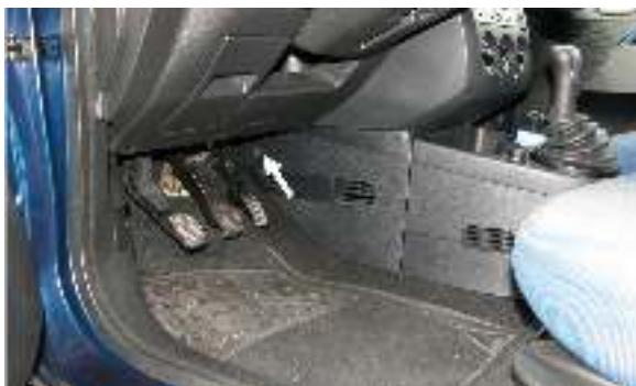
(EN) Loosen the screw and move the filter chamber cover to the left
