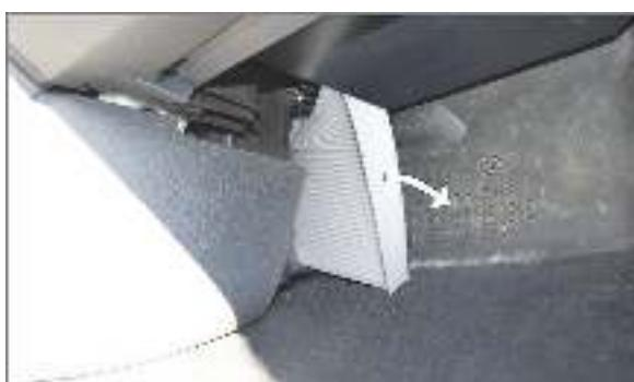
Gently remove the old filter, put in the new one and close the cover of the filter chamber attached in the kit
