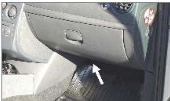
The filter is located under the glove compartment
