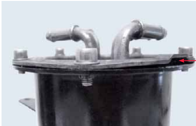
Figure 1: This housing cover (KX 178) was deformed by being opened and/or closed incorrectly.
