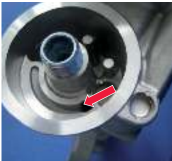
Figure 1: View of the flange on the engine side with the anti-drain back plate
