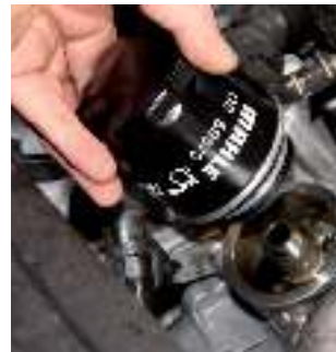
Figure 3: When loosening the old filter, make sure that no engine oil gets onto the belt drive or into the alternator.
