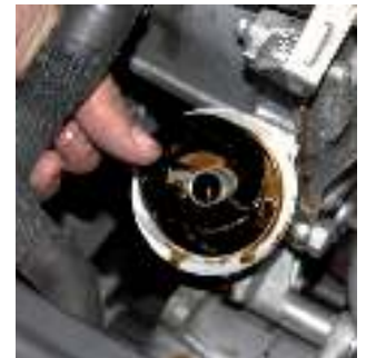
Figure 4: The old gasket can remain stuck in the flange and must always be removed.
