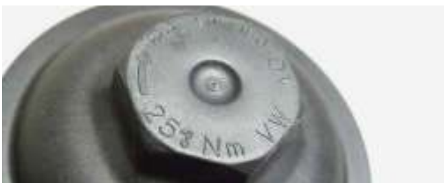
Figure 2: Torque specification on the housing cover
