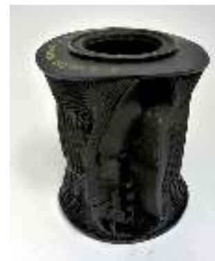
Figure 3: Oil filter insert deformed/torn as a result of overheating
