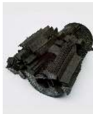
Figure 2: Disintegrated oil filter insert
