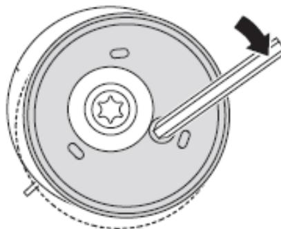
**Fig. 3 Variante 2 - Extraer el pasador tras montar la correa**
