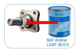
Clean the axle stub from all dirt and pollution. To avoid rust after mounting, always use SKF Antifret (LGAF 3E/0.5) on the stub axle before mounting the bearing.
