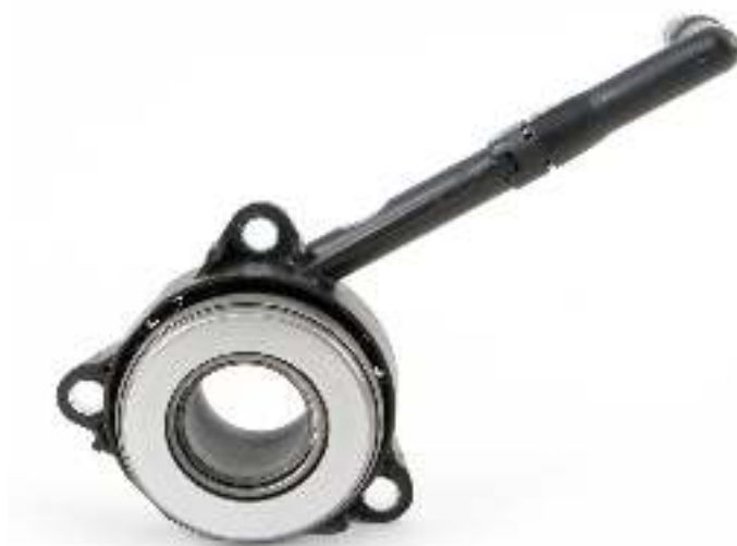
Air must be removed from the concentric slave cylinder 510 0177 10 in accordance with a specific procedure
