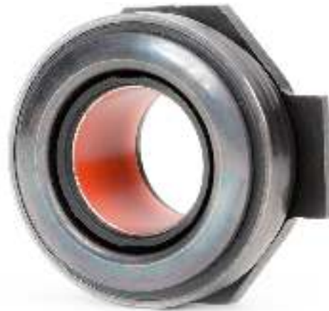
Fig. 3: Release bearings with PTFE housing must not be lubricated
