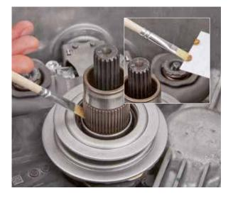
Wet the bearing seat of the transmission input shaft with a drop of transmission oil around the entire circumference
