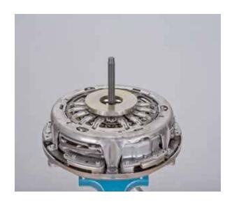
• Insert the adapter into the pressure plate
