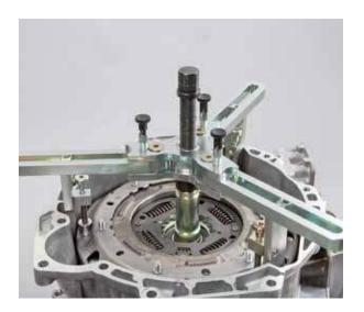
• Screw the thumb screws into the hooks by hand
