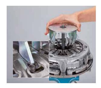
• Initially, only turn the pressure nut onto the spindle until it is touching the pressure piece
