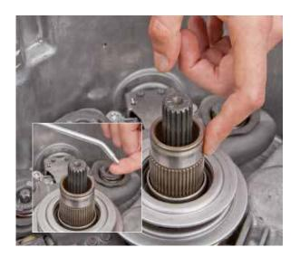
Attach the handles and place the clutch onto the hollow shaft. Turning slightly ensures that the gear teeth of clutch plate K2 and the hollow shaft mesh with each other
