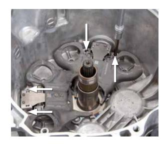
• Remove both lever actuators
