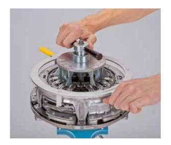
• Disassemble the pressure nut, pressure piece and return ring
