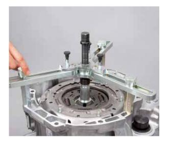
• Tighten three hexagon-socket head screws on the puller
