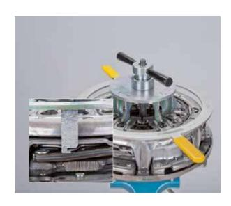
• Turn the return ring anti-clockwise (in the direction of the arrow on the ring) and hold at the stop
