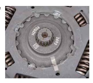
• Insert the retaining ring such that the gap in the ring is positioned centrally in relation to the plastic pin
