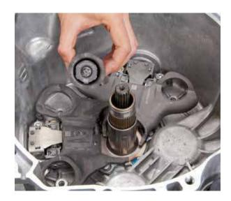
• The middle four digits on the return spring and the last four digits on the lever actuator must be identical
