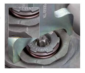
Place the special open-ended spanner (KL-0500-8010) on the housing of the return spring and turn it until the markings are aligned
