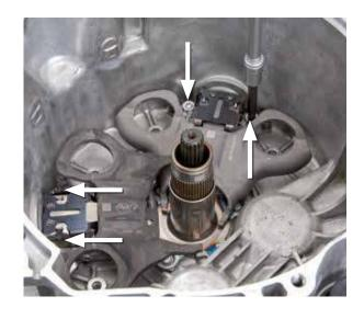
• Remove the transport fasteners from the two lever actuators
