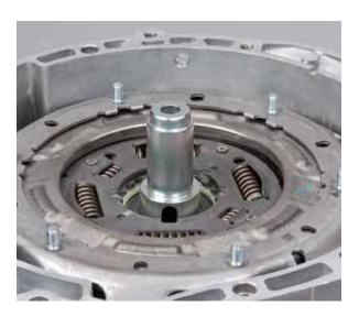
Mount three threaded bolts (KL-0500-6021 or KL-0500-6022) with collar nuts on the transmission bell housing
