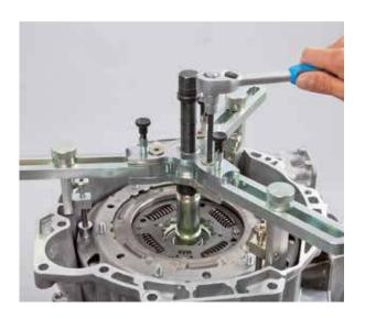
• Disconnect the clutch package by turning the spindle onto the hollow shaft
