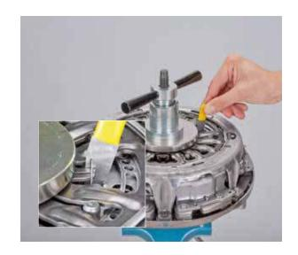
• Release and unscrew the pressure nut
