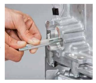
• Insert the unlocking key with the marking facing upwards into the lever actuator for K1
