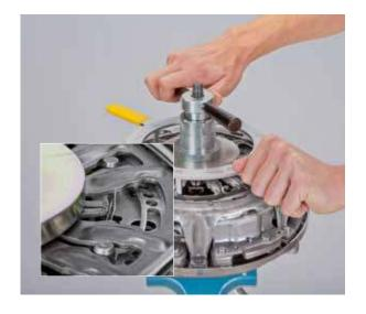
• Fit the tabs on transport fastener K1 in position using the fixing pieces
