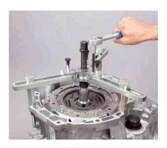
Turn the spindle via the press-in sleeve to press the clutch onto the hollow shaft; the pressing process is complete as soon as the retaining-ring groove is fully visible in one of the windows of the press-in sleeve and the amount of force required to turn the spindle increases significantly
