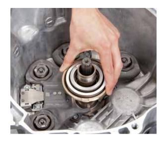
Remove the screws from the two servo motors (for K1 and K2)
