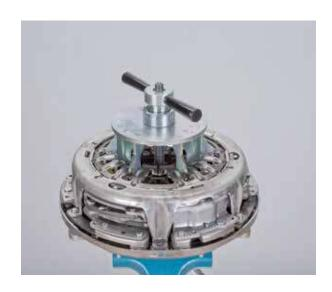
Place the large return ring for K2 (KL-0500-714) onto the double clutch and insert it into the tabs of the adjuster ring
