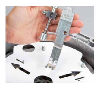
Swivel in the extractor hook and pull upwards.
