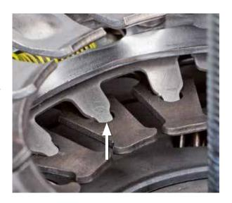
Place pressure ring K1, Ø 105 mm (KL-0500-7111), onto lever spring K1
