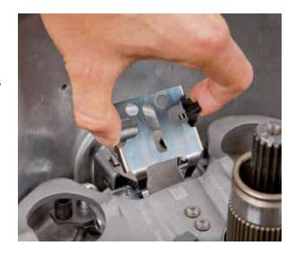
• The return spring and the lever actuator are coordinated and must therefore be assigned correctly
