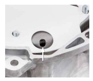
• Turn the clutch until the template is positioned as shown in the transmission bell housing
