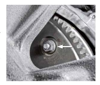
• During the removal process, insert the plugs (KL-0500-8012) into the openings of the differential
