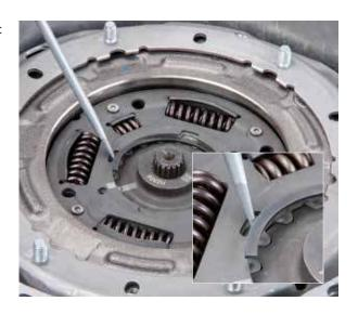
• Remove the retaining ring and clutch disc hub (K1)
