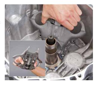
• Remove the three screws from the guiding sleeve
