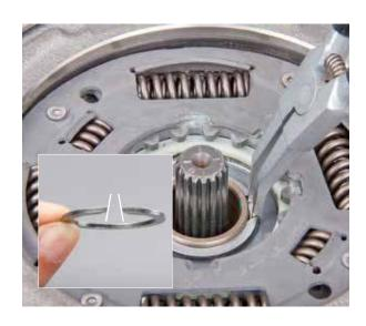
• Install the hub of the upper clutch disc (K1); the correct position is marked with a line
