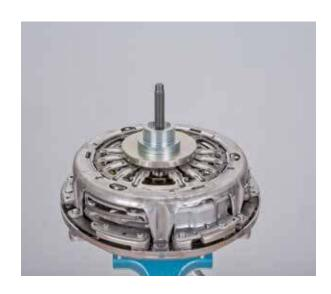
• Initially, only turn the pressure nut onto the spindle until it is touching the adapter
