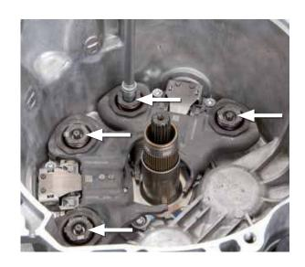
• Unscrew the mounting screws of the lever actuators
