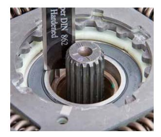
Place the pressure sleeve (KL-0500-8211) on the bearing inner ring of the clutch package
