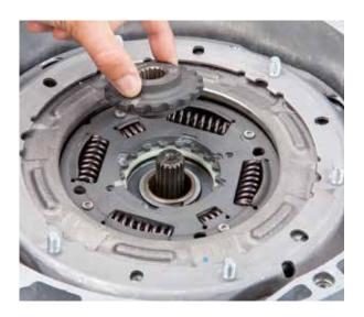
Using the snap ring pliers (KL-0192-12), remove the retaining ring from the hollow shaft; the ring is usually damaged in the process and must be replaced
