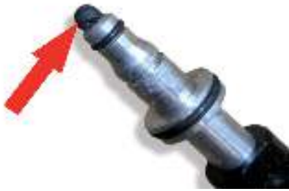
Image 4: If the old seal is not removed, it can get pressed into the CSC and block the tube
