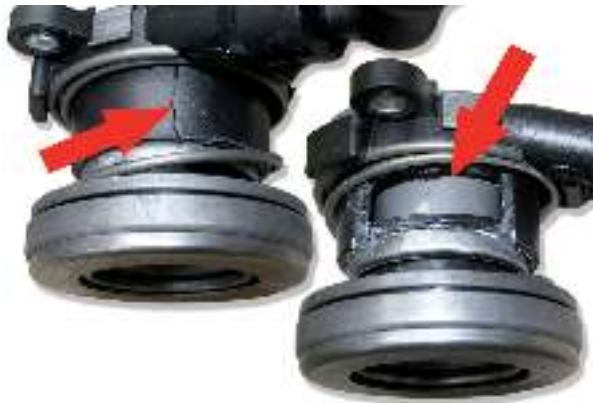
Image 5: CSC damaged by improper installation
