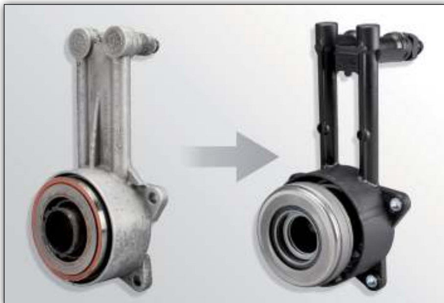
Image 1: Item replacement from a metal to plastic design
