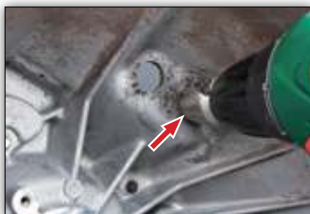
Image 5: Increasing the size of the holes
