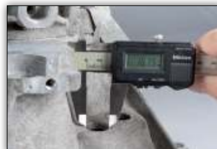
Image 2: If the diameter is smaller than 21 mm, it must be bored open to at least 21 mm, with a max. of 24 mm
