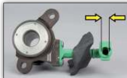
Image 4: LuK CSC 510 0137 10 hydraulic connection 12.2 mm
