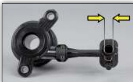
Image 3: LuK CSC 510 0098 10 hydraulic connection 11.7 mm
