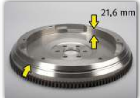
Image 2: OE no. 93186460 / 5616016 with indentation around the circumference, flywheel depth 21.6 mm
