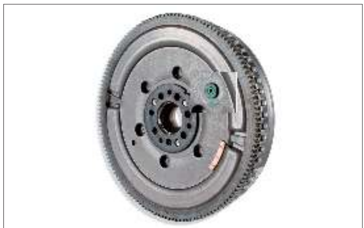
Image 1: LuK DMF with a detent pin as the transport fastener
