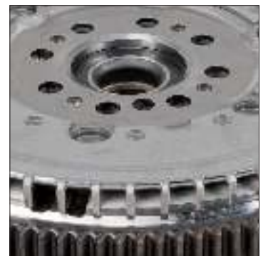
Image 2: New sensor ring design
